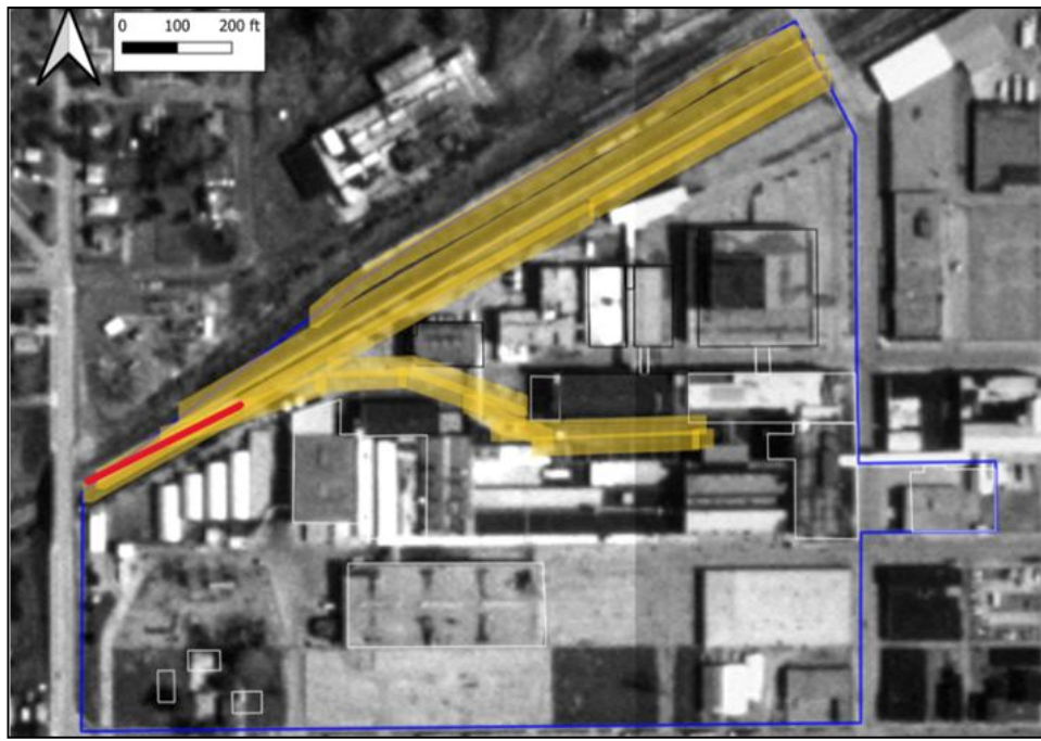
Figure 33. 1980s satellite image of the district (blue outline) with areas of past railroad sidings/spurs (yellow highlights) and extant track (red line). Accessed online through the Iowa Geographic Map Server, June 2025.
