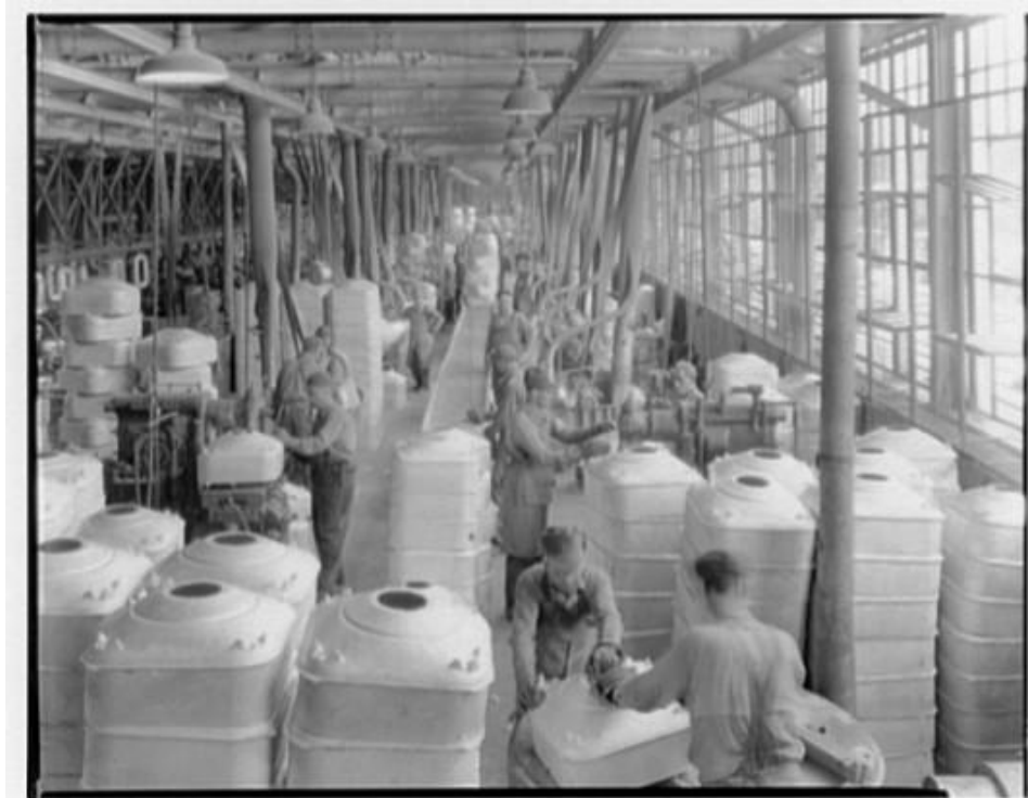
Figure 58. Grinding and Polishing Aluminum Tubs (Theodor Horydczak Collection, Library of Congress).
